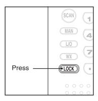
$\begin{array}{c} \text{If keys do not work, press} \\ \hline \text{LOCK} \end{array} to unlock keys. \end{array}$
